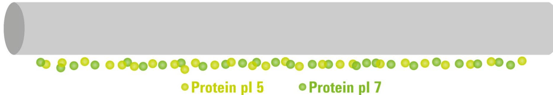
At the beginning of a CIEF run, the whole capillary (coated fused silica) is filled with:
