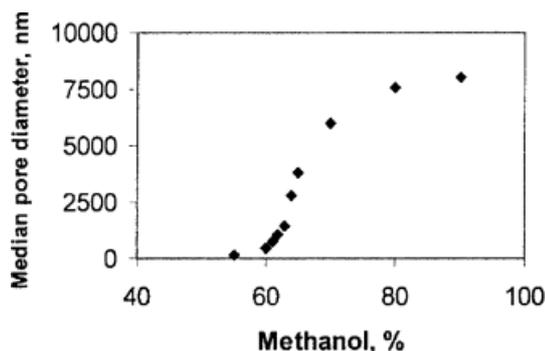
**Figure 1.** Effect of the composition of methanol-ethyl acetate mixture used as the porogenic solvent on the median pore size of poly(glycidyl methacrylate-co-ethylene dimethacrylate) monoliths. Reprinted from [4], with permission.
