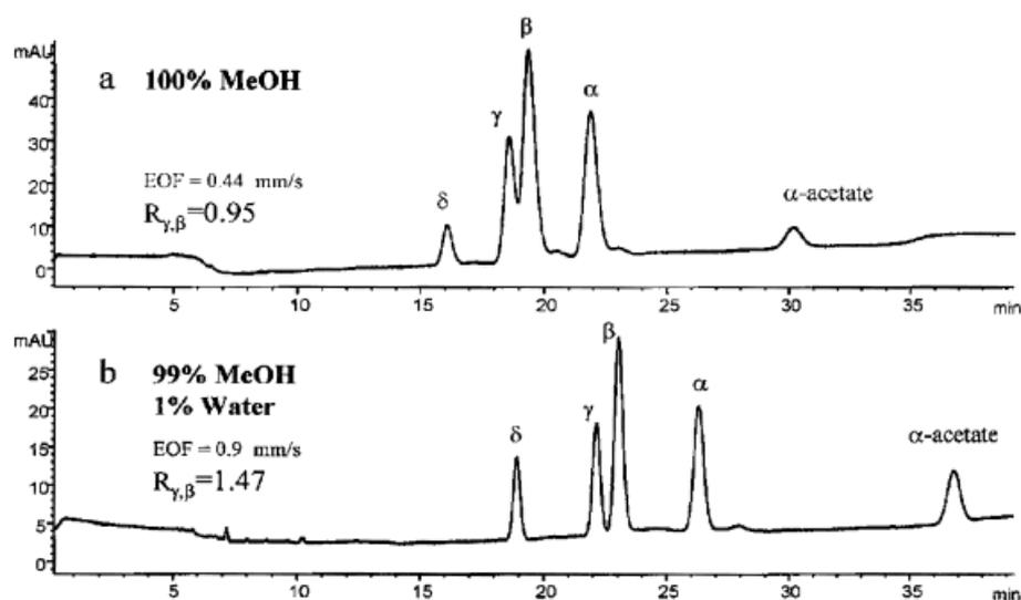
**Figure 16.** Effect of the addition of 1% water to the methanol mobile phase on the separation between  $\beta$ -,  $\gamma$ -tocopherol isomers using a  $C_{30}$  monolithic stationary phase. Reprinted from [102], with permission.
