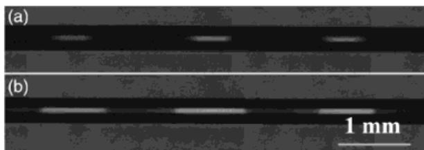
**Figure 2.** Fluorescence microscopy image of a porous (butyl methacrylate-co-ethylene dimethacrylate) monolith photografted with poly(4,4-dimethyl-2-vinylazlactone) through a mask for (a) 1 and (b) 3 min and subsequently reacted with Rhodamine 6G. Reprinted from [7], with permission.
