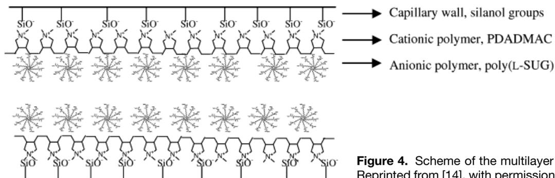
**Figure 4.** Scheme of the multilayer coating for OT-CEC. Reprinted from [14], with permission.
