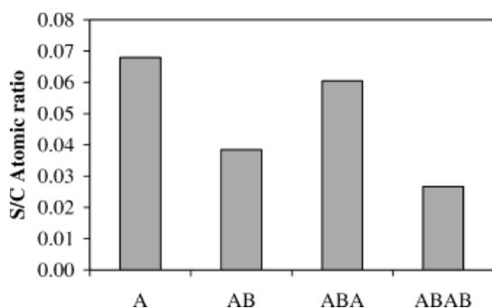
**Figure 3.** Sulfur to carbon atomic ratio for subsequently photografted layers using (A) AMPS (B) and butylacrylate. Reprinted from [6], with permission.
