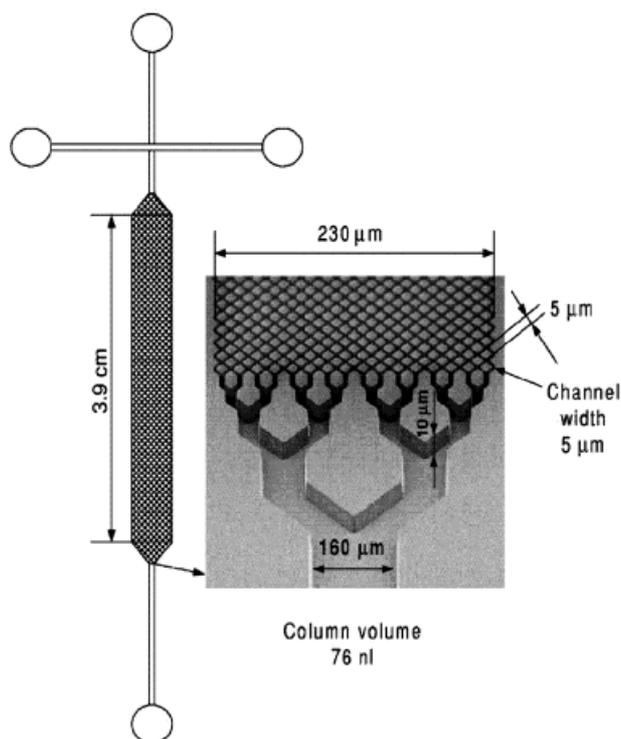
**Figure 9.** Scheme of a COMOSS column with its typical dimensions. Reprinted from [77], with permission.
