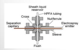
FS separation capillary 50x150 μm
