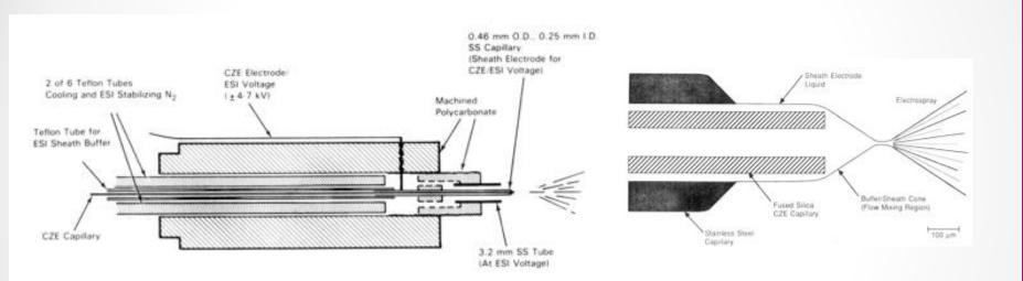
Sheath solvent delivered at 5-10  $\mu$ L/min Electrode in liquid electrical contact applying ES-voltage Inert sheath gas to protect the spray Stable and true electrospray
