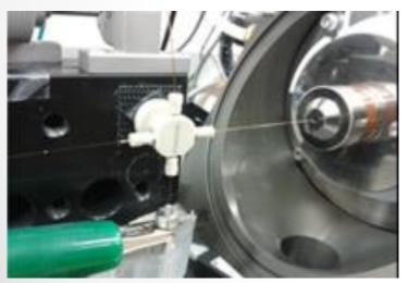
**Separation capillary**: FS 75x150 μm **Emitter capillary**: FS 200x350 μm, end etched with HF and orifice 50 μm **BGE**: 25 mM ammonium acetate, pH 4 **Sheath solvent and TE**:9/1 0.1 M acetic acid/methanol
