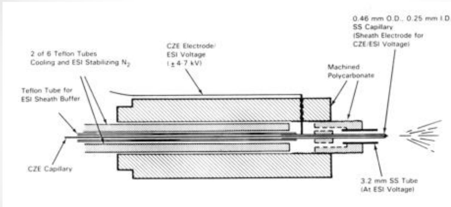
Sheath solvent delivered at 5-10  $\mu\text{L}/\text{min}$
