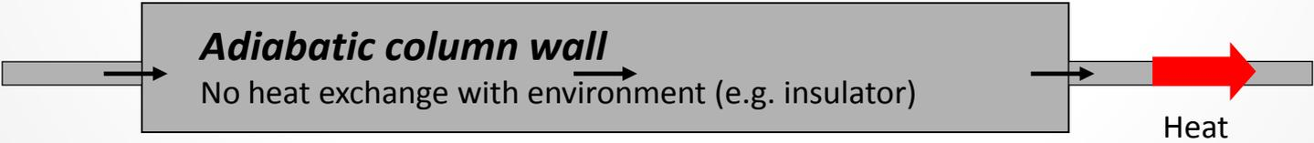
Frictional heat is released via column effluent
